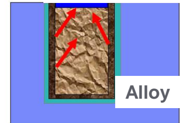
(Approach-2) Metal Cap fed from inside CuMn Seed Layer
